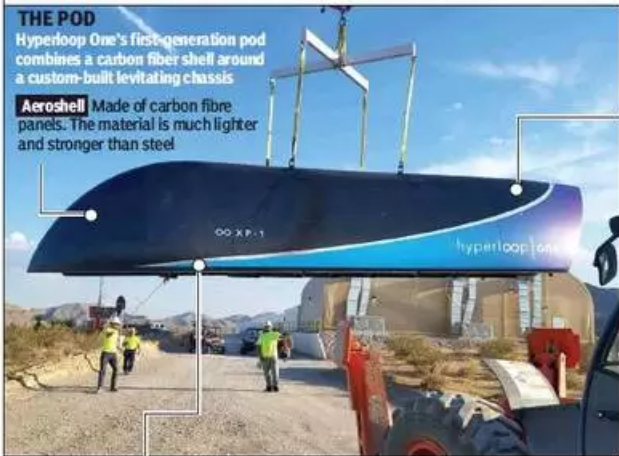
In December 2017, Hyperloop One's pod reached a top speed of over 385 kmph on its test track in the Nevada desert, north of Las Vegas. The targeted speed is 1,223 kmph
