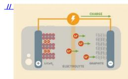
Lithium-ion batteries power many of our electronic devices. When lithiumion batteries charge, lithium ions and electrons move from the positive electrode to the negative electrode. When the battery is discharging, the opposite happens and the flow of electrons powers the device.
