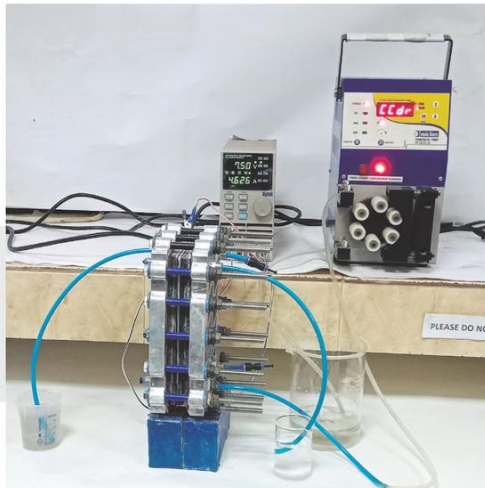
Hydrogen is produced at a rate of one litre per hour when a large electrolyser is used
