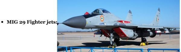
It is a twin-engine, multirole fighter jet, developed by the Soviet Russia in the 1970s. It has been upgraded since.
