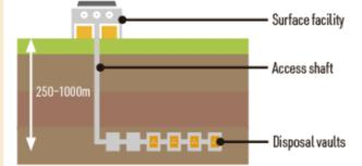
Intermediate and high level waste generate heat and greater levels of radioactivity. Most countries plan to use deep geological disposal. The rock and soil acts as a barrier to the radiation. Before this, high level waste is incorporated into glass and stored for up to fifty years to allow heat to dissipate.
