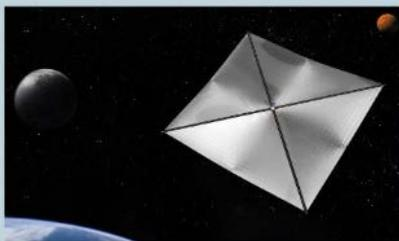
Solar sails (left) could remain in place by balancing against the pressure of light from the sun. The satellite would not be in orbit, it would actually hover in space. Such a satellite is called a "statite."
